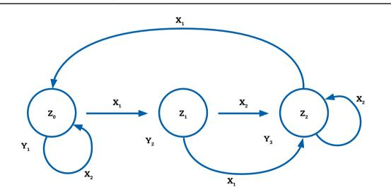
Note: The figure represents a finite state automaton with three states  $z_0$ ,  $z_1$ , and  $z_2$ , and two input variables  $x_1$  and  $x_2$ , leading to three possible output signals  $y_1$ ,  $y_2$ , and  $y_3$  depending on the reached state. Source: Funke (2001:78).
